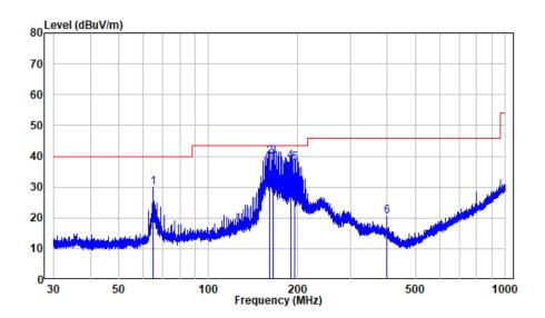
Site : chamber Condition: 3m HORIZONTAL Job No. : RA230330-15712E-RF Test Mode: 5G WIFI Transmitting
