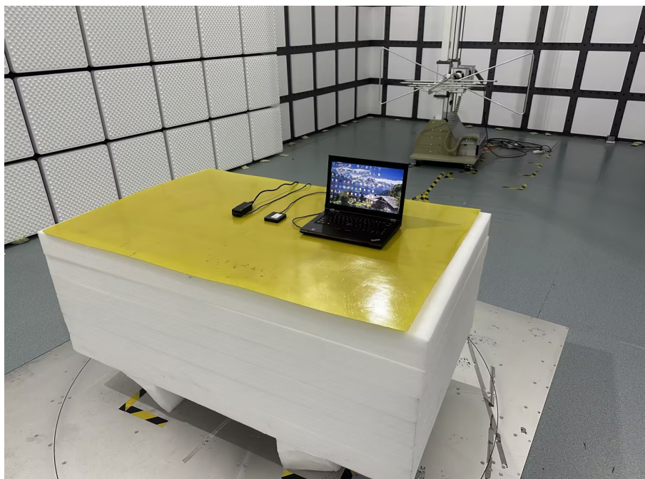
Photo of Radiated Emission Measurement (Below 1G)
