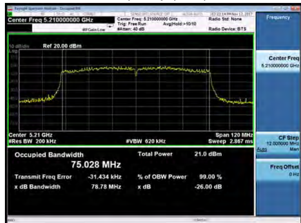
U-NII-1, 802.11ac HT80 Carrier frequency (MHz): 5210
