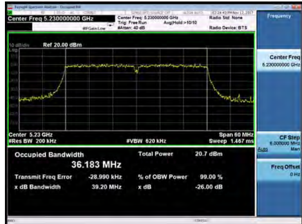
U-NII-1, 802.11ac HT80 Carrier frequency (MHz): 5210
