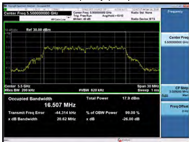
U-NII-2C, 802.11ac HT20 Carrier frequency (MHz): 5580
