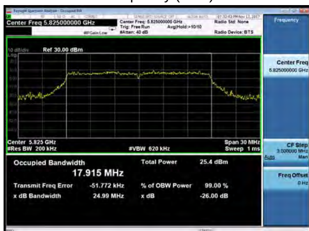
U-NII-3, 802.11ac HT20 Carrier frequency (MHz): 5825
