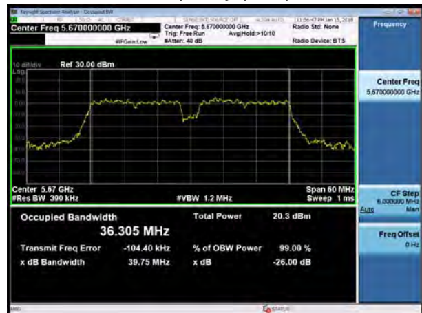
U-NII-2C, 802.11ac HT40 Carrier frequency (MHz): 5670
