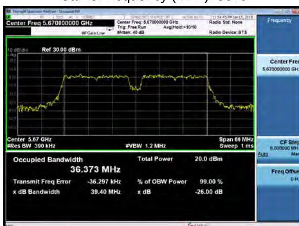
U-NII-2C, 802.11n HT40 Carrier frequency (MHz): 5670
