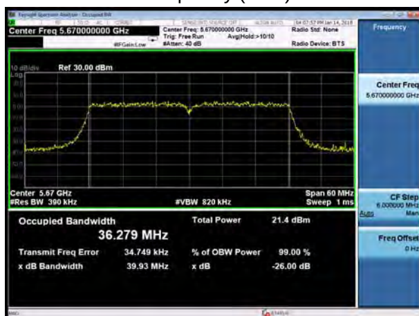
U-NII-2C, 802.11ac HT40 Carrier frequency (MHz): 5670
