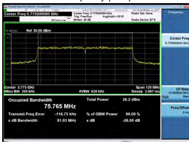
U-NII-3, 802.11ac HT80 Carrier frequency (MHz): 5775
