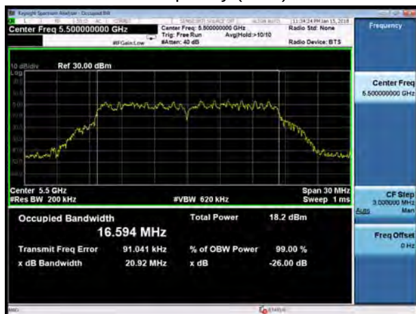
U-NII-2C, 802.11n HT20 Carrier frequency (MHz): 5580
