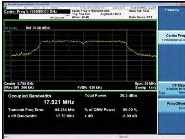
U-NII-3, 802.11ac HT20 Carrier frequency (MHz): 5825
