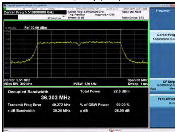
U-NII-2C, 802.11ac HT40 Carrier frequency (MHz): 5550
