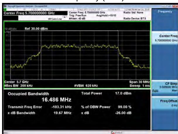
U-NII-2C, 802.11ac HT20 Carrier frequency (MHz): 5700
