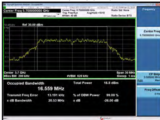
U-NII-2C, 802.11ac HT20 Carrier frequency (MHz): 5700
