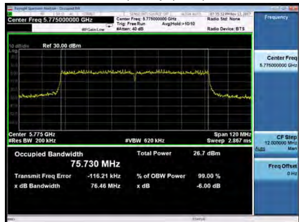
U-NII-3, 802.11ac HT80 Carrier frequency (MHz): 5775
