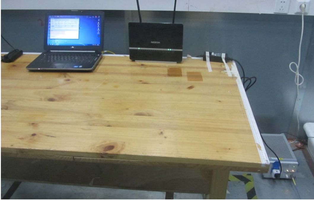
Picture 3 Conducted Emission Test Setup
