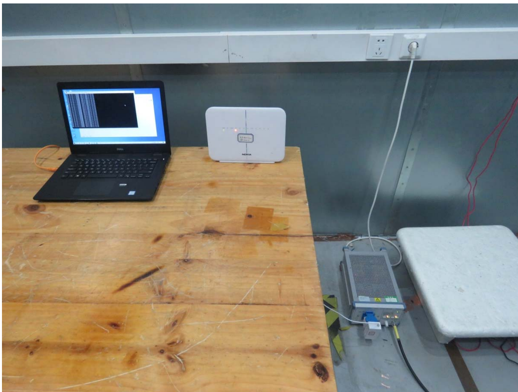
Picture 2 Conducted Emission Test Setup
