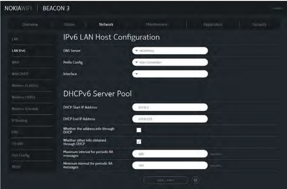
Figure 23 LAN IPv6 network window
