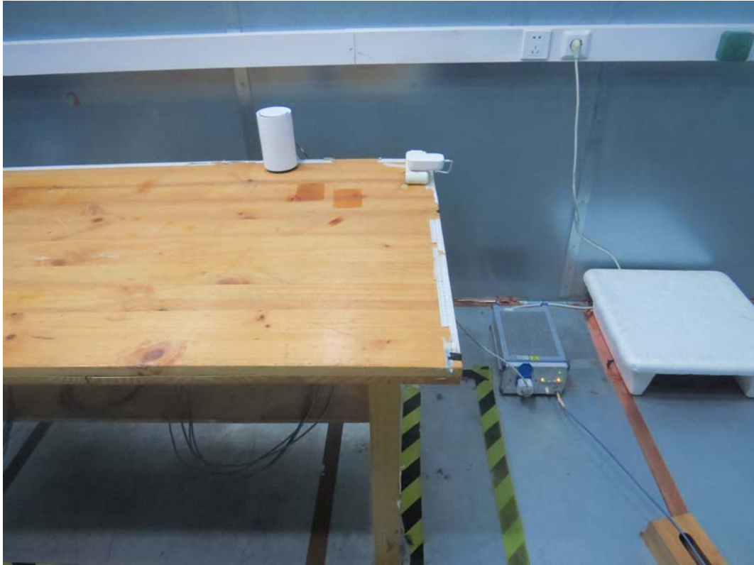
Conducted Emission Test Setup
