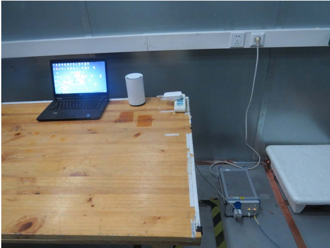
Picture 3 Conducted Emission Test Setup
