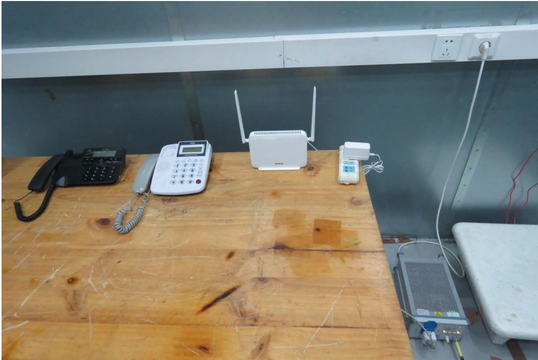
Picture 2 Conducted Emission Test Setup
