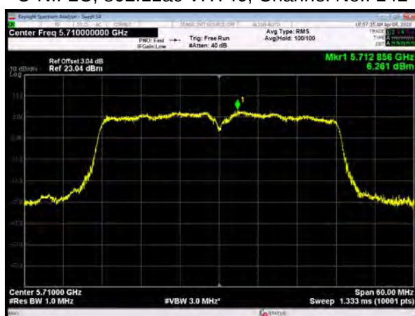
U-NII-2C, 802.11ac VHT80, Channel No.: 138
