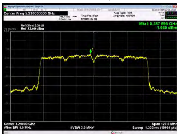
U-NII-2A, 802.11ac VHT80, Channel No.: 58
