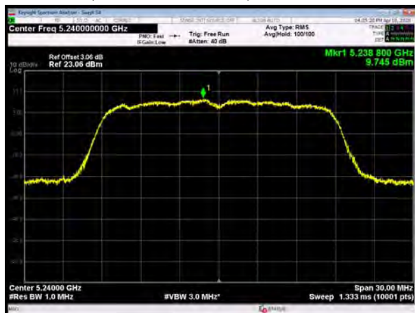
U-NII-1, 802.11ac VHT20, Channel No.: 48
