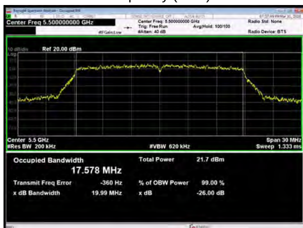
U-NII-2C, 802.11ac VHT20 Carrier frequency (MHz): 5600
