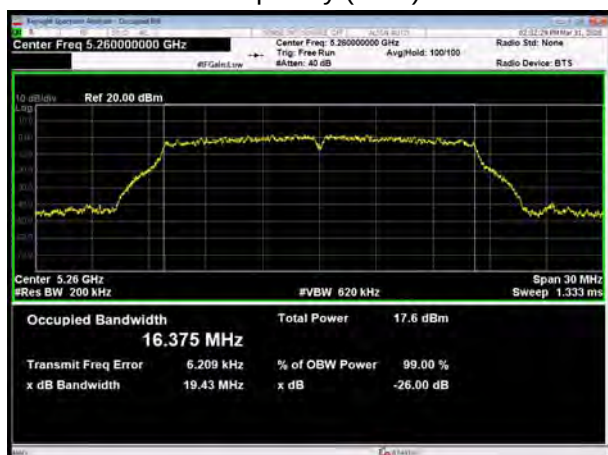
U-NII-2A, 802.11a Carrier frequency (MHz): 5300
