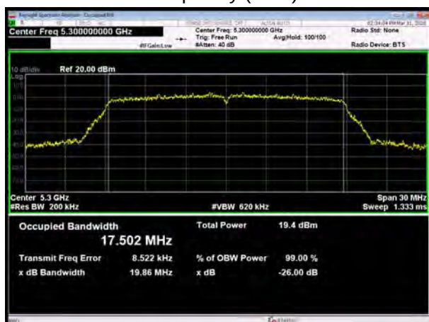
U-NII-2A, 802.11n HT20 Carrier frequency (MHz): 5320
