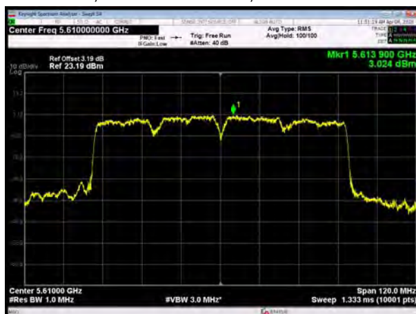
U-NII-2C, 802.11ac VHT80, Channel No.: 122
