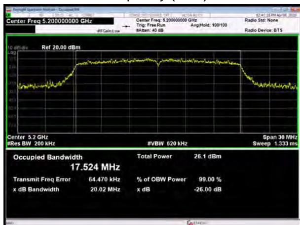
U-NII-1, 802.11n HT20 Carrier frequency (MHz): 5240
