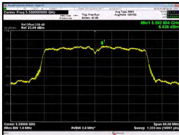
U-NII-2C, 802.11ac VHT40, Channel No.: 118
