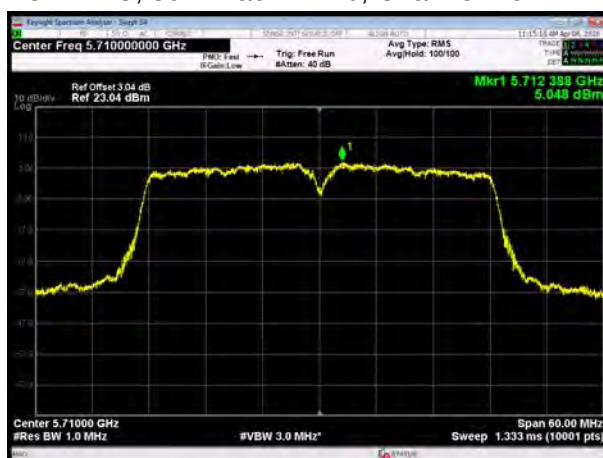
U-NII-2C, 802.11ac VHT80, Channel No.: 138
