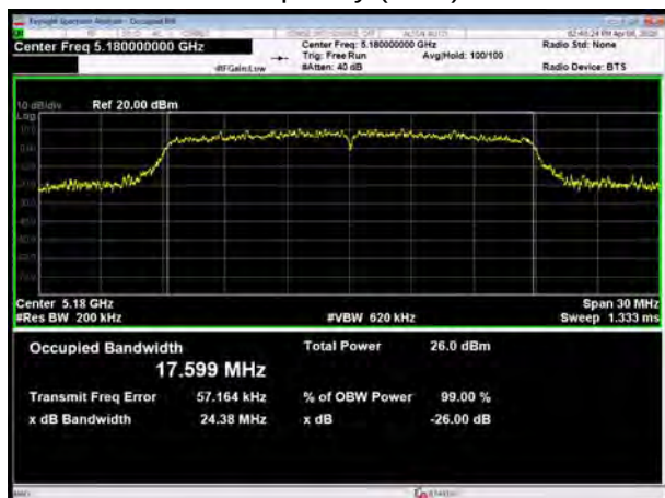
U-NII-1, 802.11n HT20 Carrier frequency (MHz): 5200
