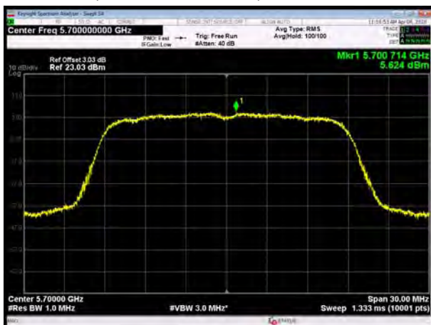
U-NII-2C, 802.11ac VHT20, Channel No.: 144
