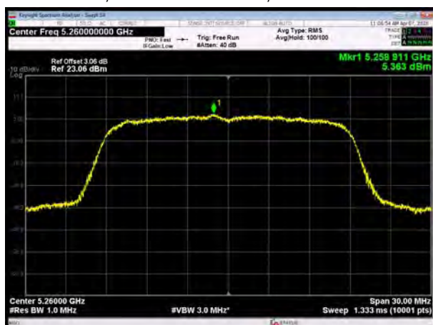
U-NII-2A, 802.11ac VHT20, Channel No.: 60
