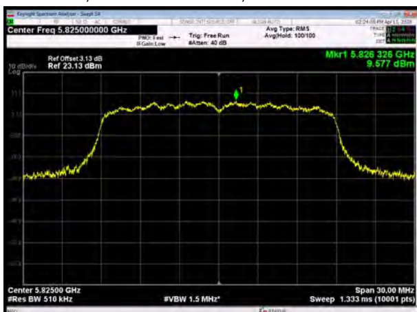
U-NII-3, 802.11ac VHT20, Channel No.: 165
