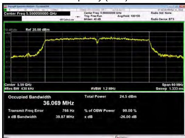
U-NII-2C, 802.11ac VHT40 Carrier frequency (MHz): 5670
