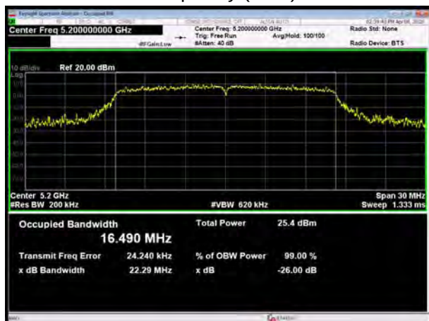
U-NII-1, 802.11a Carrier frequency (MHz): 5240
