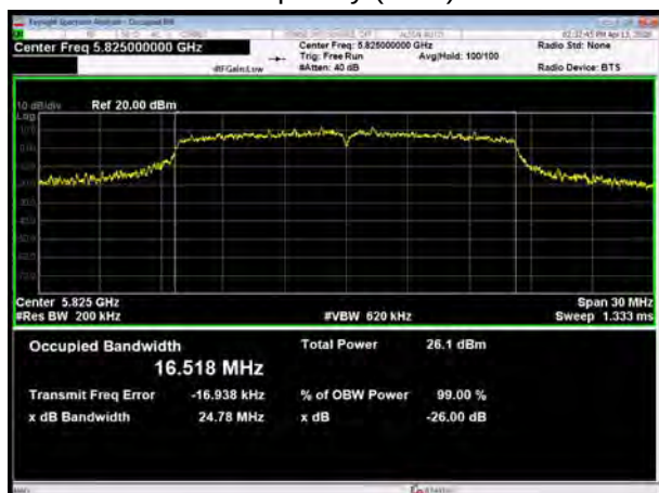
U-NII-3, 802.11a Carrier frequency (MHz): 5825
