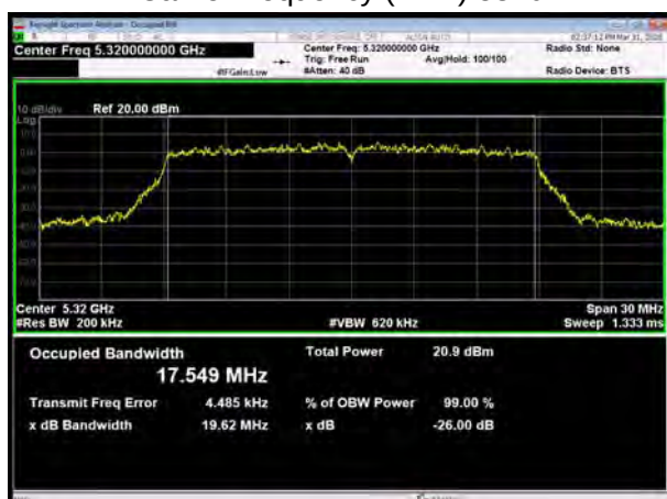
U-NII-2A, 802.11ac VHT80 Carrier frequency (MHz): 5290
