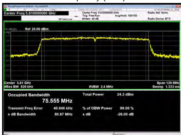
U-NII-2C, 802.11ac VHT80 Carrier frequency (MHz): 5690
