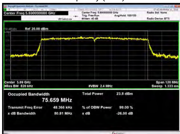
U-NII-2C, 802.11ac VHT40 Carrier frequency (MHz): 5710
