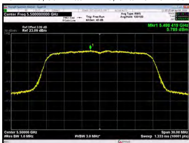
U-NII-2C, 802.11ac VHT20, Channel No.: 120
