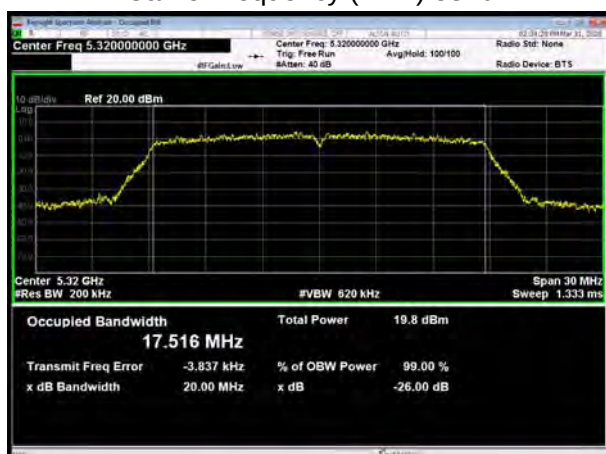
U-NII-2A, 802.11n HT20 Carrier frequency (MHz): 5320
