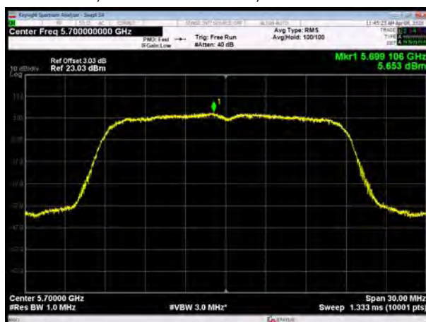
U-NII-2C, 802.11ac VHT20, Channel No.: 144
