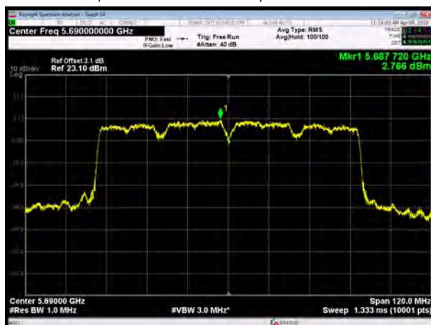
U-NII-2C, 802.11ac VHT80, Channel No.: 138
