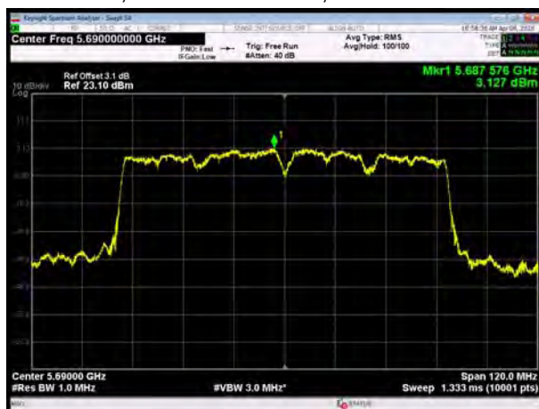
U-NII-2C, 802.11ac VHT80, Channel No.: 138
