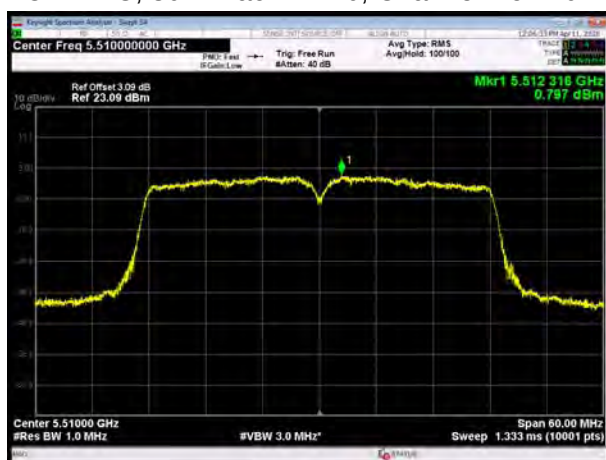
U-NII-2C, 802.11ac VHT40, Channel No.: 118
