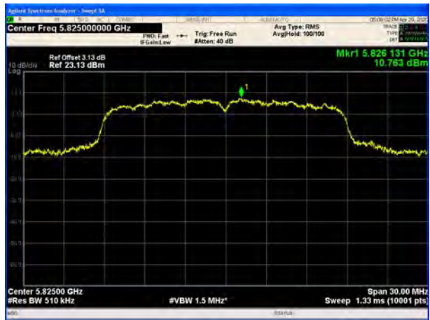
U-NII-3, 802.11ac VHT20, Channel No.: 165
