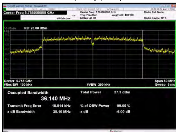
U-NII-3, 802.11ac VHT40 Carrier frequency (MHz): 5755
