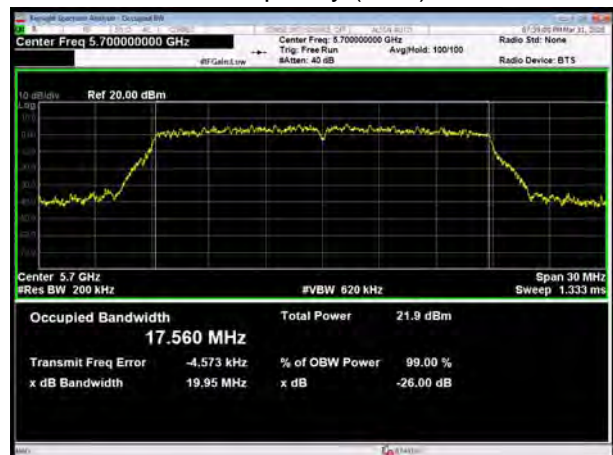
U-NII-2C, 802.11ac VHT20 Carrier frequency (MHz): 5720
