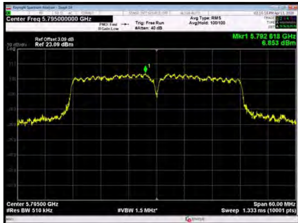
U-NII-3, 802.11ac VHT80, Channel No.: 155
