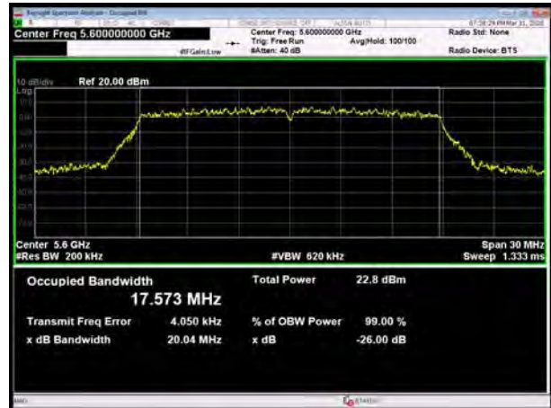
U-NII-2C, 802.11ac VHT20 Carrier frequency (MHz): 5700
