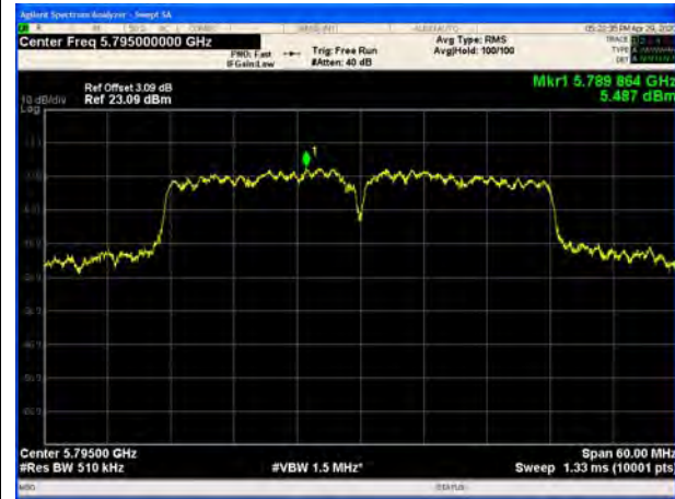
U-NII-3, 802.11ac VHT40, Channel No.: 159
