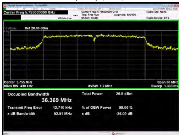
U-NII-3, 802.11ac VHT40 Carrier frequency (MHz): 5755
