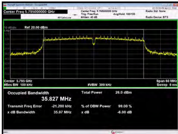
U-NII-3, 802.11ac VHT40 Carrier frequency (MHz): 5755
