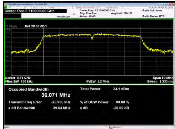
U-NII-2C, 802.11ac VHT40 Carrier frequency (MHz): 5710
