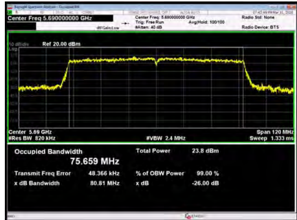
U-NII-2C, 802.11ac VHT40 Carrier frequency (MHz): 5710
