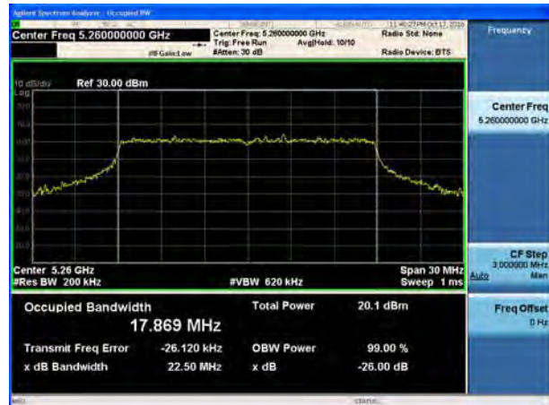
U-NII-2A, 802.11ac HT20 26 dB bandwidth Carrier frequency (MHz): 5300
