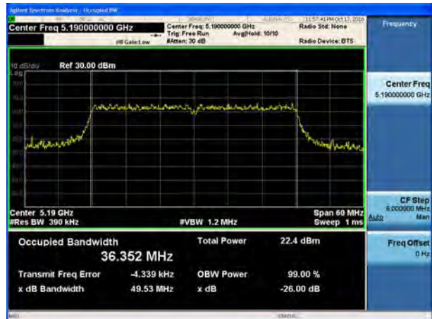
U-NII-1, 802.11ac HT40 26 dB bandwidth Carrier frequency (MHz): 5230
