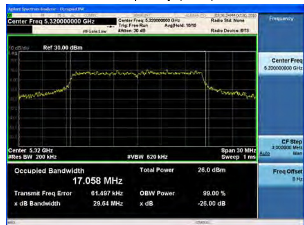
U-NII-2A, 802.11a 26 dB bandwidth Carrier frequency (MHz):5320
