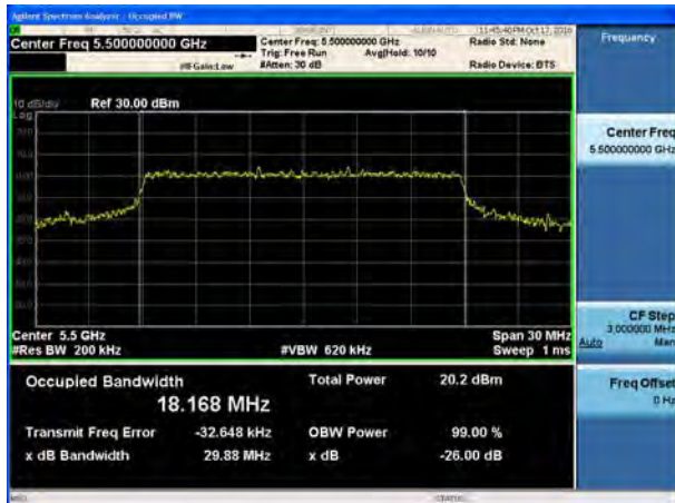
U-NII-2C, 802.11ac HT20 26 dB bandwidth Carrier frequency (MHz): 5580
