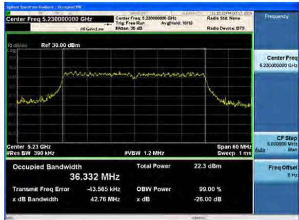
U-NII-1, 802.11n HT40 26 dB bandwidth Carrier frequency (MHz): 5230
