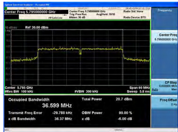
U-NII-3, 802.11n HT40 6 dB bandwidth Carrier frequency (MHz): 5795
