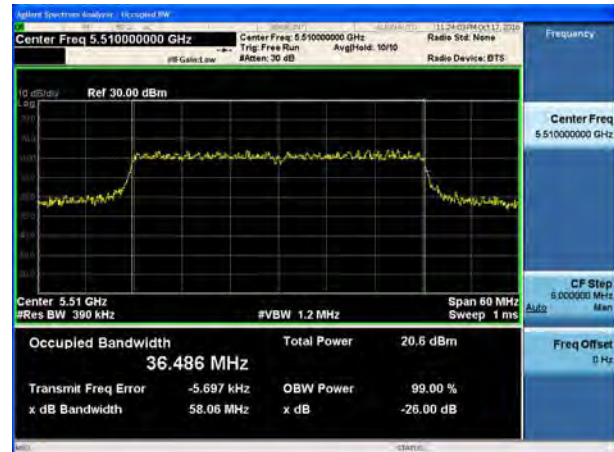
U-NII-2C, 802.11n HT40 26 dB bandwidth Carrier frequency (MHz): 5550
