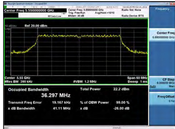
U-NII-2C, 802.11n HT40 26 dB bandwidth Carrier frequency (MHz): 5670
