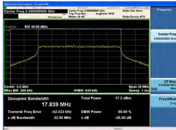
U-NII-2C, 802.11n HT20 26 dB bandwidth Carrier frequency (MHz): 5580
