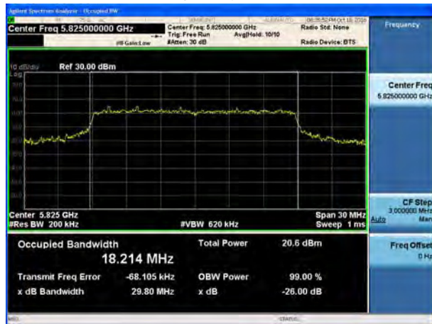
U-NII-3, 802.11n HT20 99% bandwidth Carrier frequency (MHz): 5825
