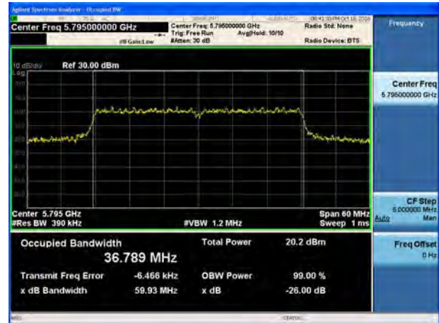
U-NII-3, 802.11n HT40 99% bandwidth Carrier frequency (MHz): 5795
