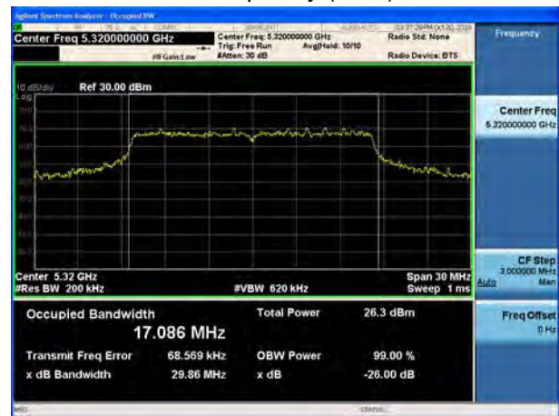
U-NII-2A, 802.11a 26 dB bandwidth Carrier frequency (MHz):5320
