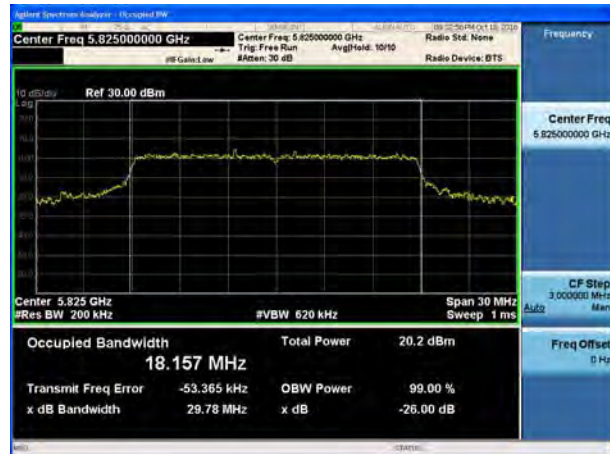
U-NII-3, 802.11ac HT20 99% bandwidth Carrier frequency (MHz): 5825
