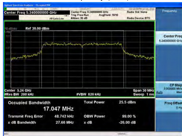
U-NII-1, 802.11a 26 dB bandwidth Carrier frequency (MHz):5240
