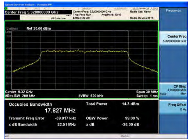
U-NII-2A, 802.11n HT20 26 dB bandwidth Carrier frequency (MHz):5320
