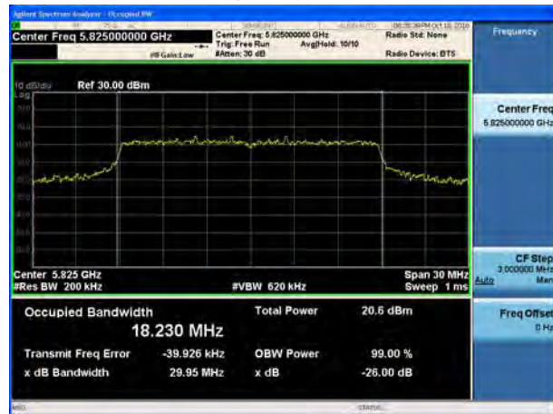
U-NII-3, 802.11n HT20 99% bandwidth Carrier frequency (MHz): 5825
