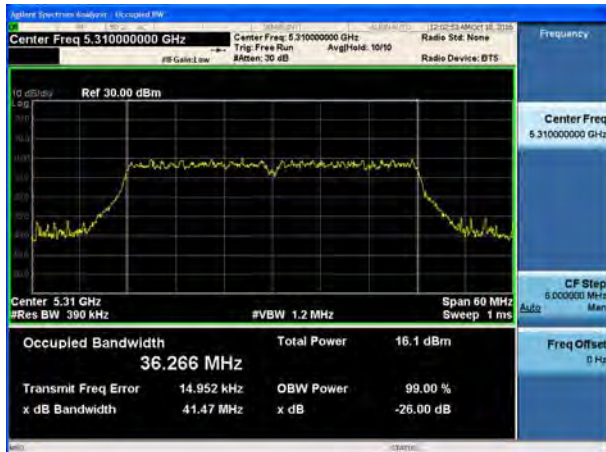
U-NII-2A, 802.11 ac HT40 26 dB bandwidth Carrier frequency (MHz): 5310
