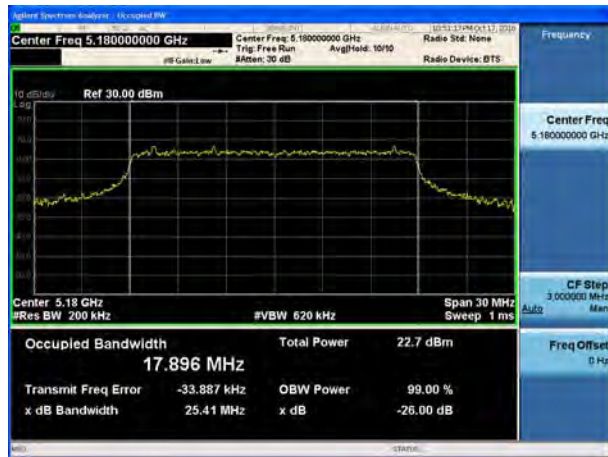
U-NII-1, 802.11n HT20 26 dB bandwidth Carrier frequency (MHz): 5200
