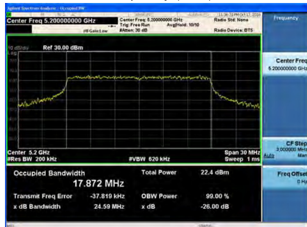
U-NII-1, 802.11ac HT20 26 dB bandwidth Carrier frequency (MHz): 5240
