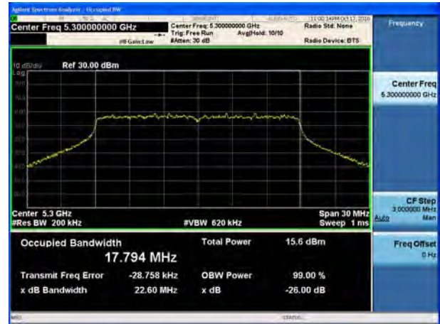
U-NII-2A, 802.11n HT20 26 dB bandwidth Carrier frequency (MHz):5320
