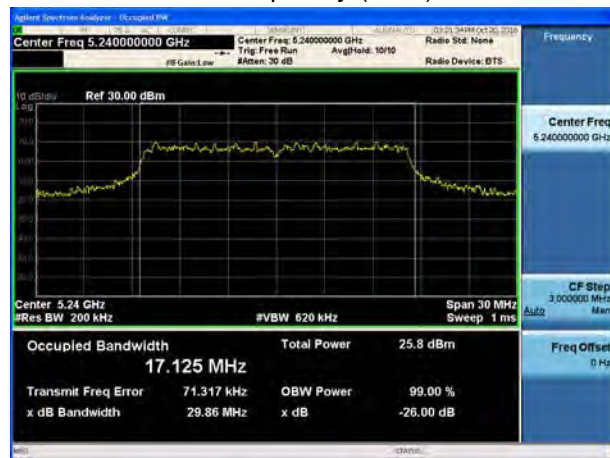
U-NII-1, 802.11a 26 dB bandwidth Carrier frequency (MHz):5240
