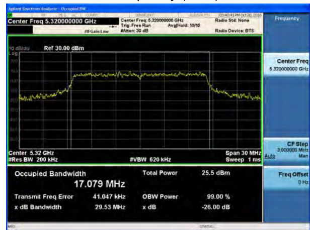
U-NII-2A, 802.11a 26 dB bandwidth Carrier frequency (MHz):5320
