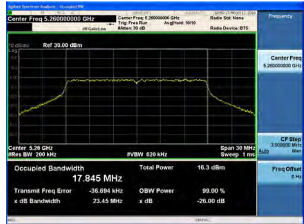
U-NII-2A, 802.11n HT20 26 dB bandwidth Carrier frequency (MHz): 5300
