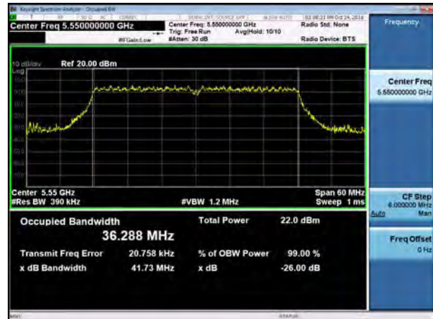
U-NII-2C, 802.11 ac HT40 26 dB bandwidth Carrier frequency (MHz): 5670
