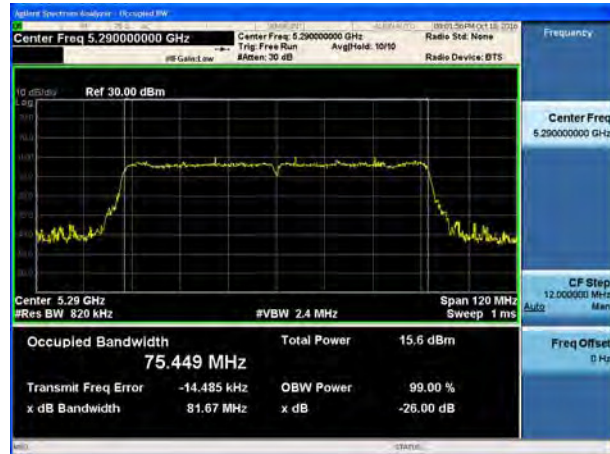
U-NII-2A, 802.11ac HT80 26 dB bandwidth Carrier frequency (MHz): 5290
