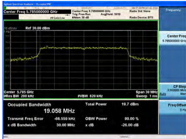
U-NII-3, 802.11n HT20 99% bandwidth Carrier frequency (MHz): 5825
