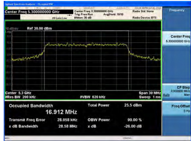
U-NII-2A, 802.11a 26 dB bandwidth Carrier frequency (MHz):5320
