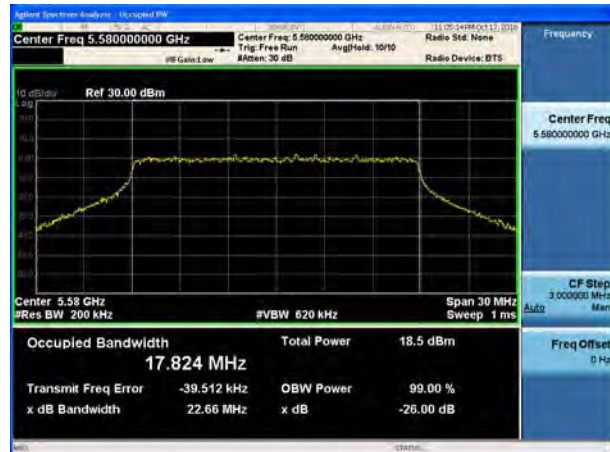
U-NII-2C, 802.11n HT20 26 dB bandwidth Carrier frequency (MHz): 5700
