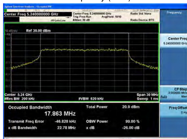
U-NII-1, 802.11ac HT20 26 dB bandwidth Carrier frequency (MHz): 5240
