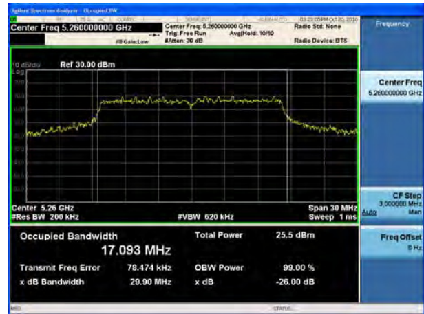
U-NII-2A, 802.11a 26 dB bandwidth Carrier frequency (MHz): 5300
