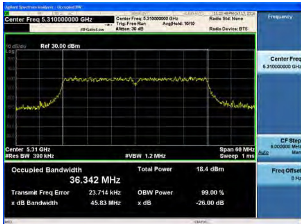
U-NII-2A, 802.11n HT40 26 dB bandwidth Carrier frequency (MHz): 5310
