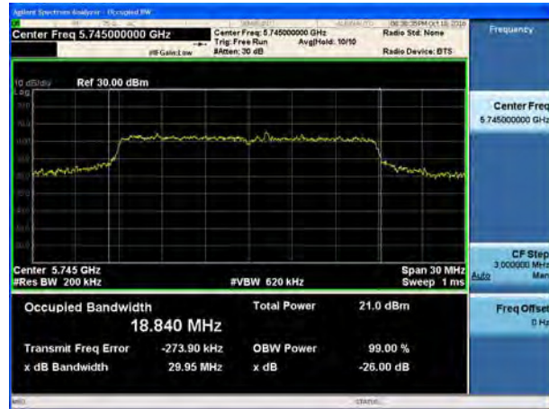
U-NII-3, 802.11n HT20 99% bandwidth Carrier frequency (MHz): 5785
