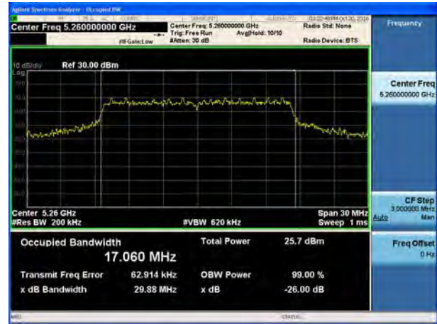
U-NII-2A, 802.11a 26 dB bandwidth Carrier frequency (MHz): 5300
