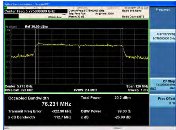
U-NII-3, 802.11ac HT80 99% bandwidth Carrier frequency (MHz): 5775
