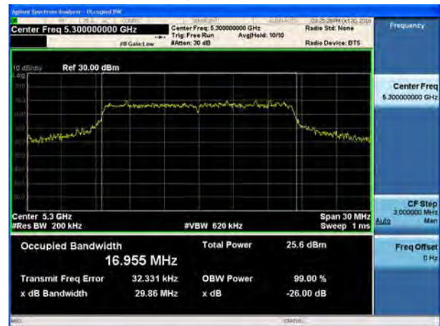
U-NII-2A, 802.11a 26 dB bandwidth Carrier frequency (MHz):5320
