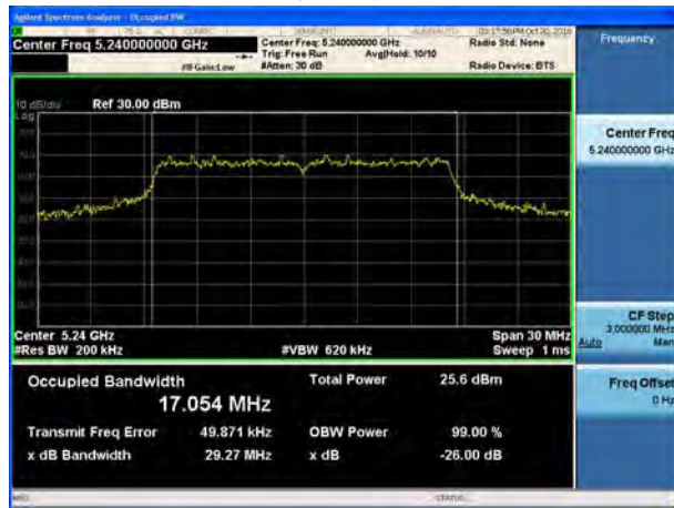
U-NII-1, 802.11a 26 dB bandwidth Carrier frequency (MHz):5240
