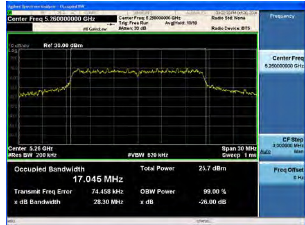
U-NII-2A, 802.11a 26 dB bandwidth Carrier frequency (MHz): 5300
