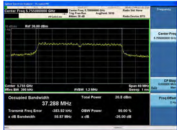
U-NII-3, 802.11n HT40 99% bandwidth Carrier frequency (MHz): 5795
