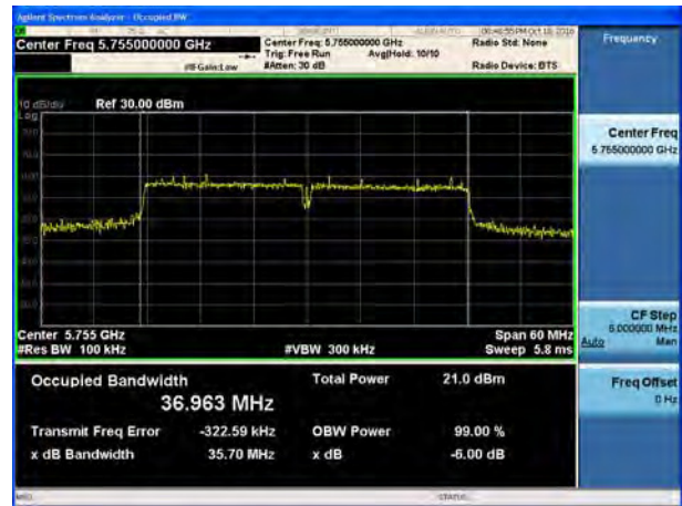
U-NII-3, 802.11n HT40 6 dB bandwidth Carrier frequency (MHz): 5795
