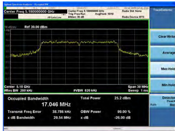
U-NII-1, 802.11a 26 dB bandwidth Carrier frequency (MHz): 5200
