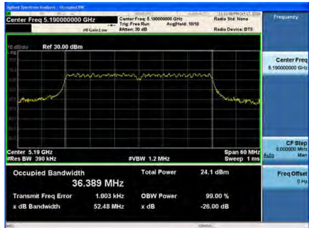
U-NII-1, 802.11n HT40 26 dB bandwidth Carrier frequency (MHz): 5230
