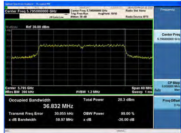
U-NII-3, 802.11n HT40 99% bandwidth Carrier frequency (MHz): 5795
