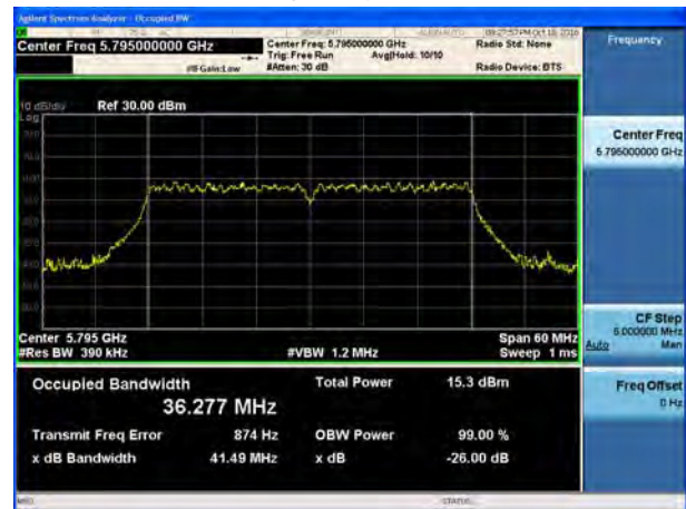
U-NII-3, 802.11ac HT80 99% bandwidth Carrier frequency (MHz): 5775
