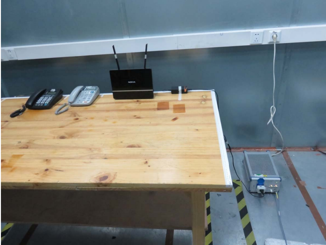
Picture 3 Conducted Emission Test Setup
