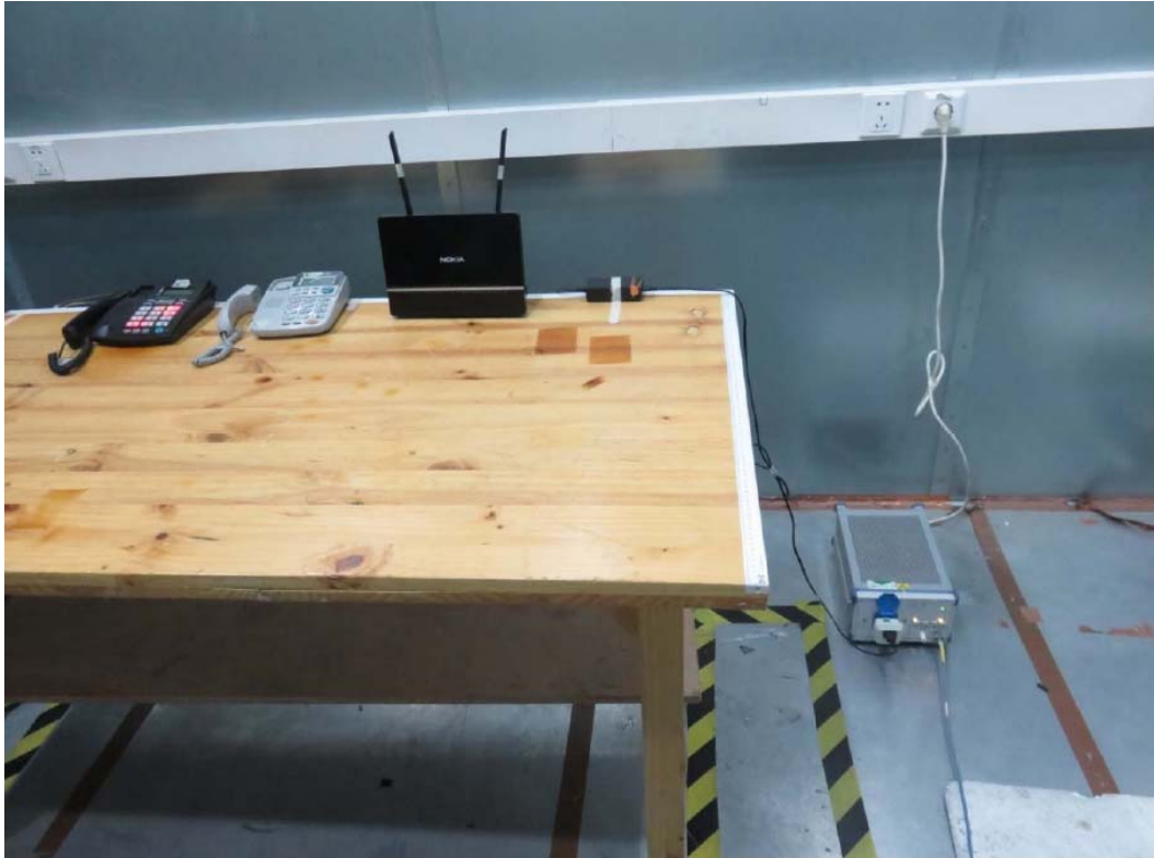
Picture 3 Conducted Emission Test Setup
