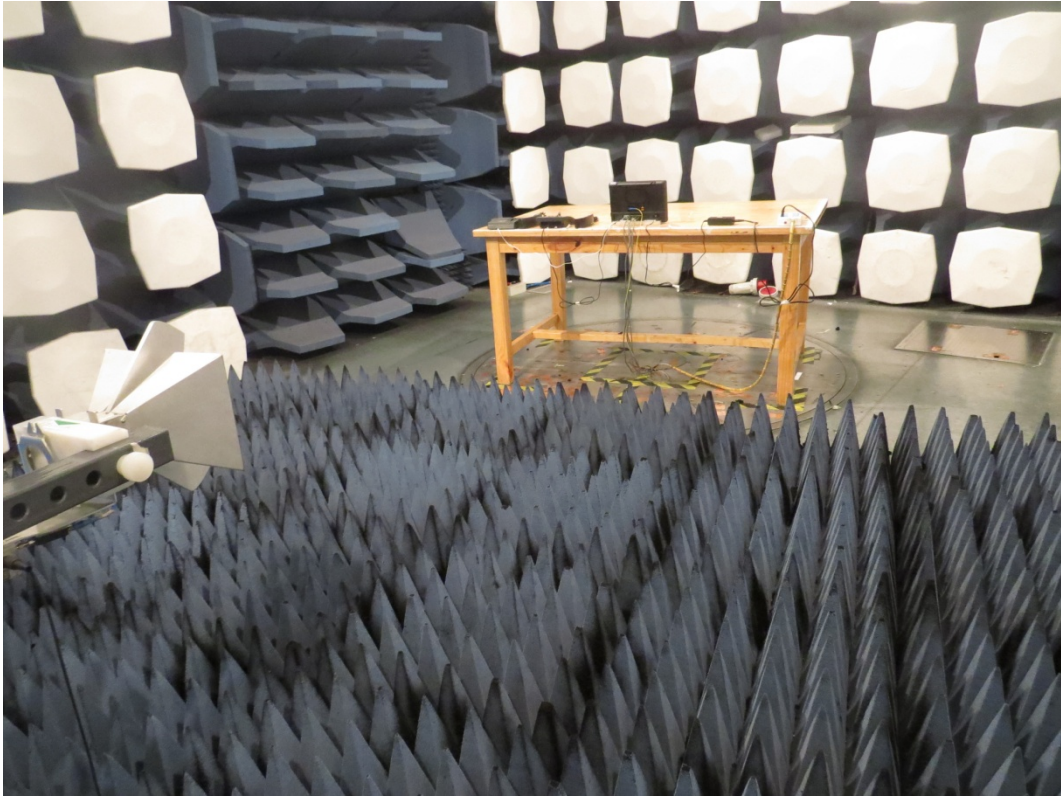
b: Above 1GHz Radiated Emission Test Setup
