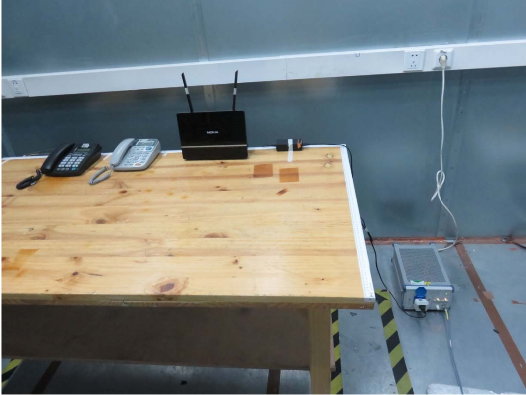
Picture 3 Conducted Emission Test Setup
