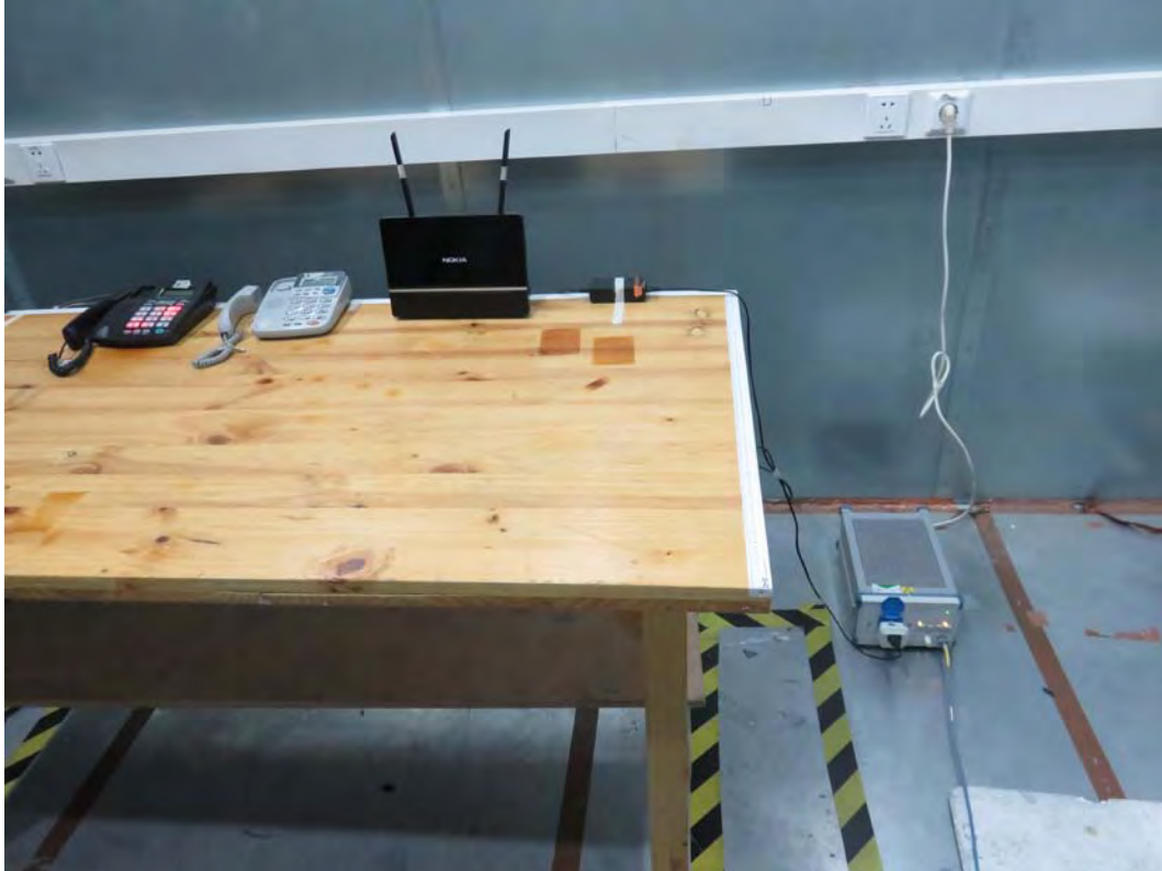
Picture 3 Conducted Emission Test Setup
