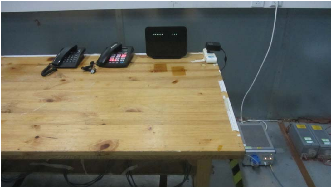
Picture 3 Conducted Emission Test Setup
