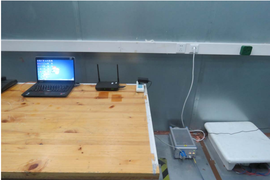
Picture 3 Conducted Emission Test Setup
