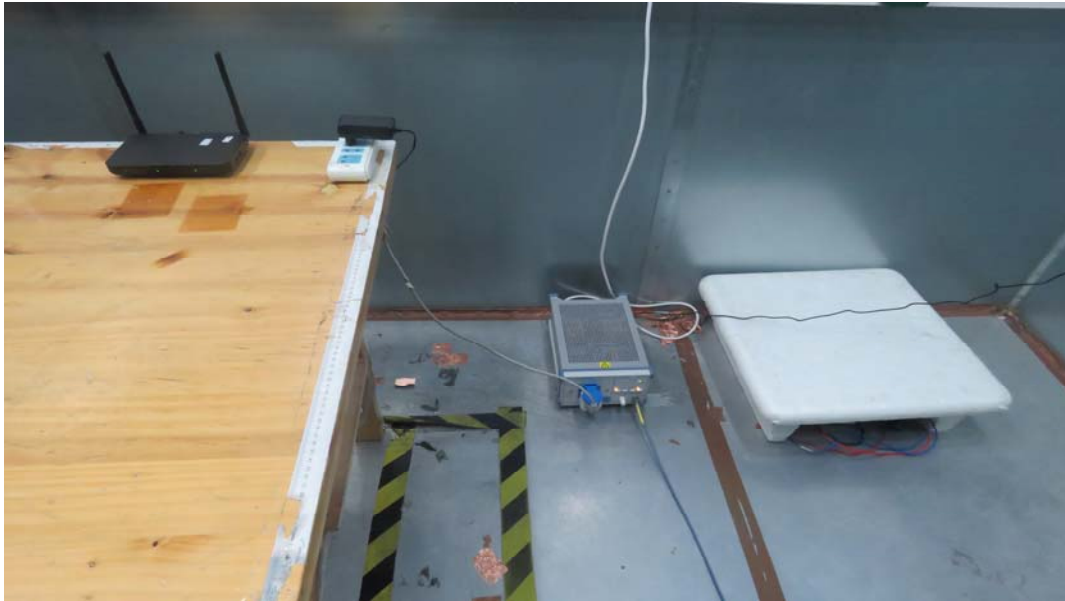
Picture 3 Conducted Emission Test Setup
