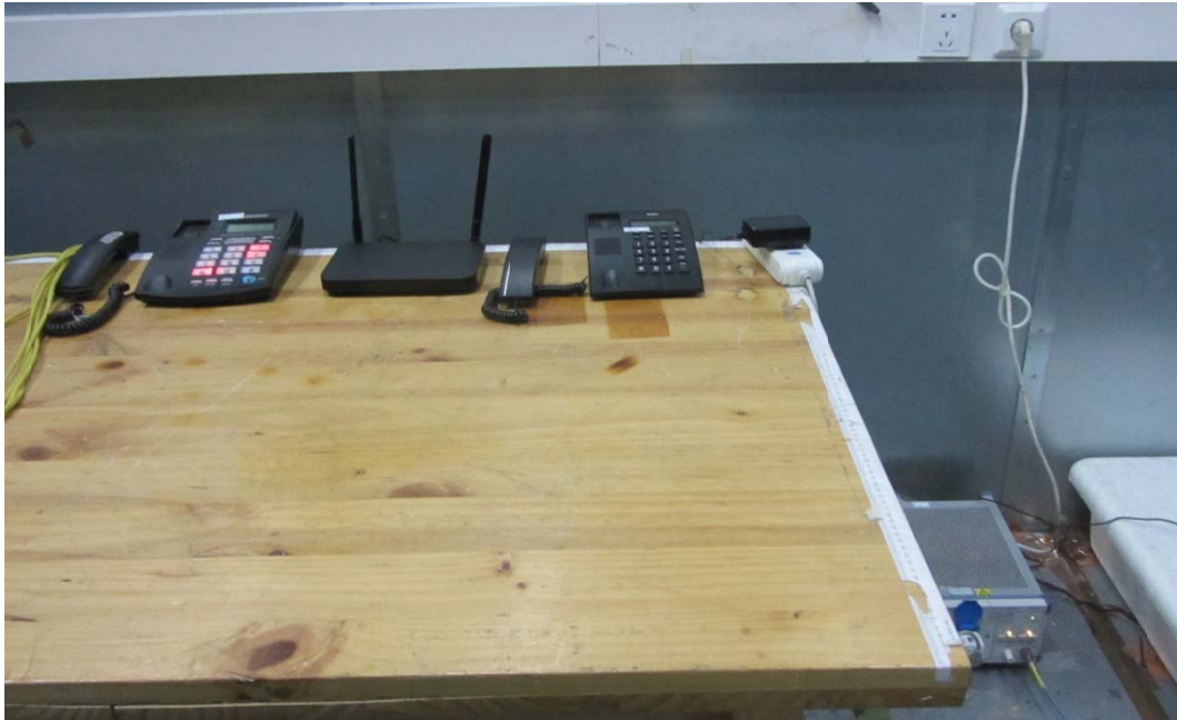
Picture 3 Conducted Emission Test Setup
