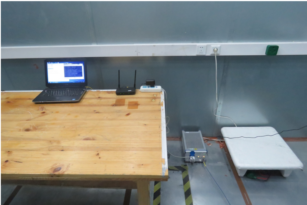
Conducted Emission Test Setup
