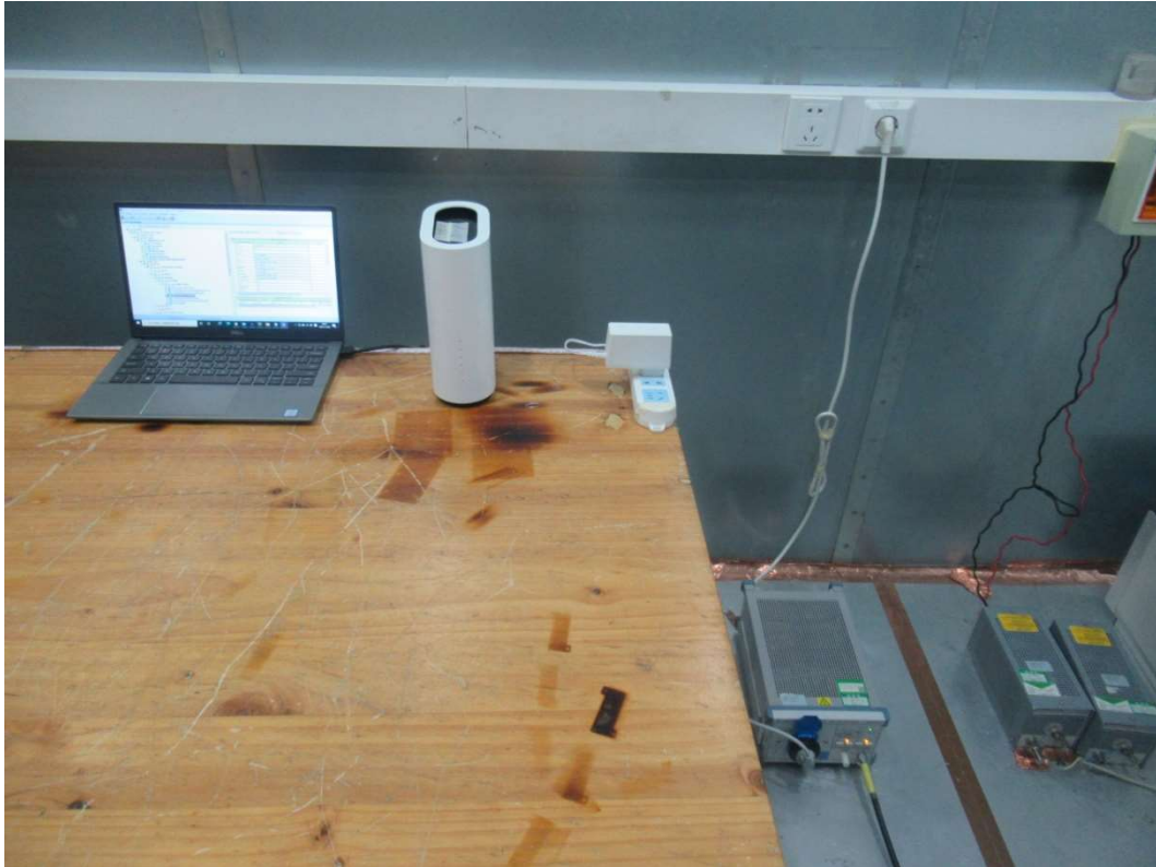
Picture 2 Conducted Emission Test Setup
