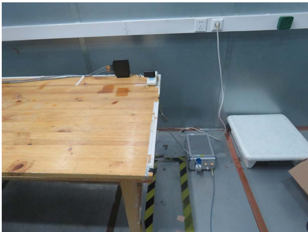
Picture 3 Conducted Emission Test Setup
