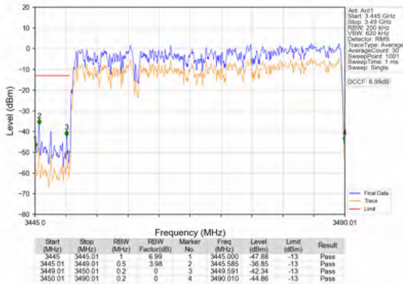
n78e_15kHz_SISO_NTNV_40MHz_DFT-s-OFDM PI/2 BPSK_3470.01MHz_Outer_Full
