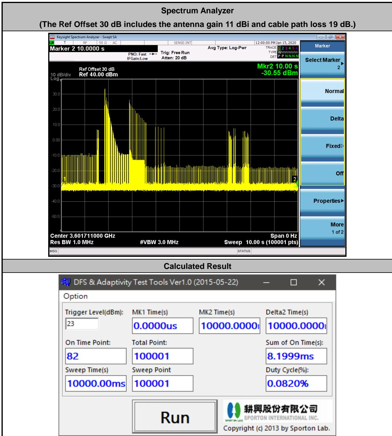
The sum of On Time (aggregated time from marker 1 to 2): 8.19ms < 20s, Pass.
