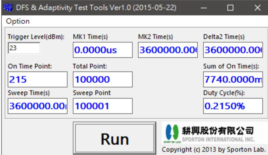
The sum of On Time (aggregated time from marker 1 to 2): 7.74s < 20s, Pass.
