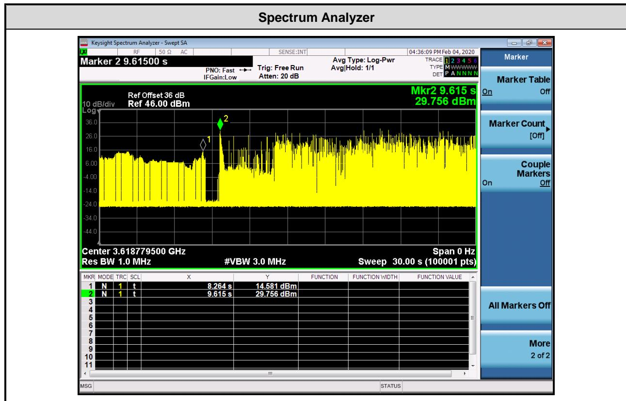
Note : The Ref Offset 36 dB includes the antenna gain 11 dBi and cable path loss 25 dB.
