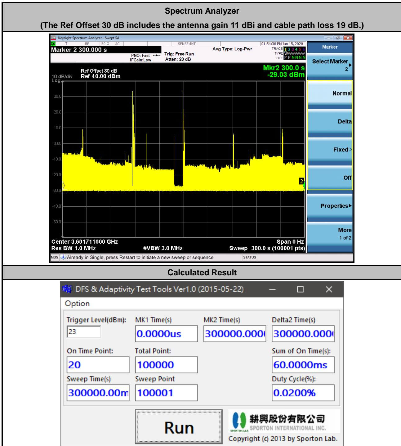
The sum of On Time (aggregated time from marker 1 to 2): 60ms < 20s, Pass.
