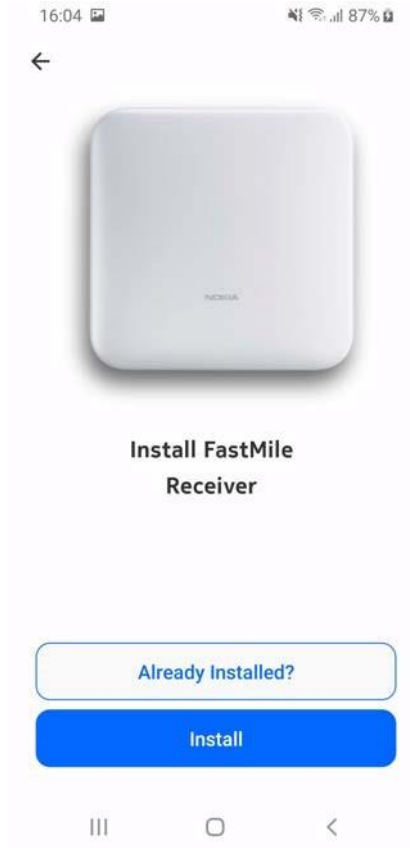
Figure 23 Screen showing the Already Installed option for unit managed by the Nokia Altiplano FastMile Controller through NETCONF
