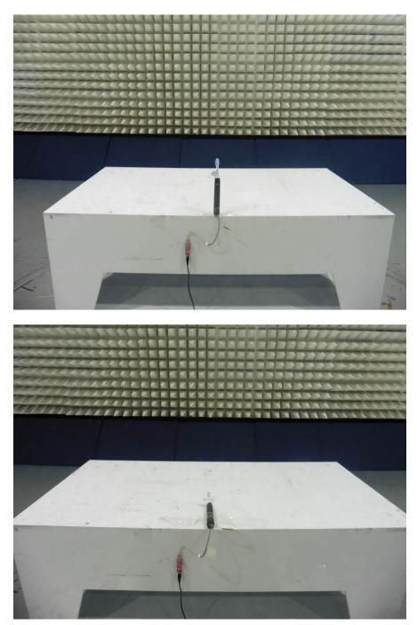
Electromagnetic Radiated Disturbance Setup Photograph
