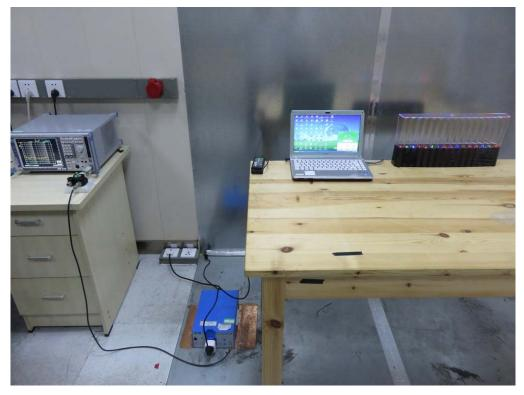
FCC RADIATED EMISSION TEST SETUP
