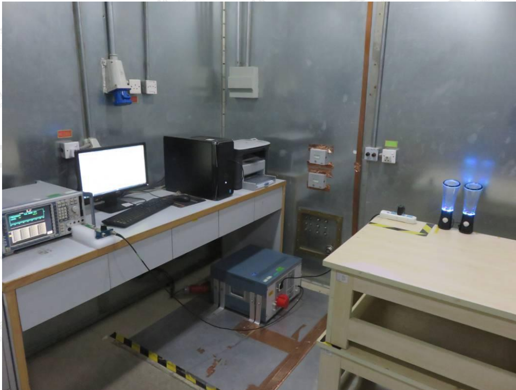
FCC RADIATED EMISSION TEST SETUP
