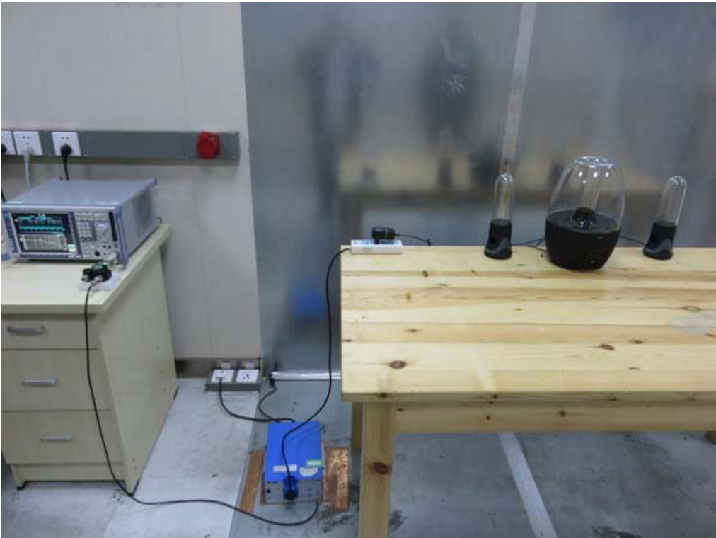
FCC RADIATED EMISSION TEST SETUP
