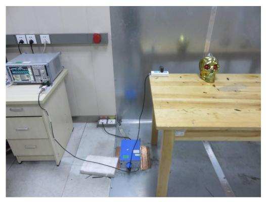
FCC RADIATED EMISSION TEST SETUP
