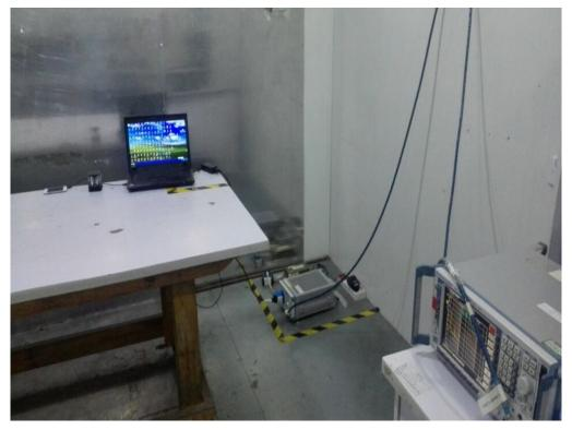
FCC RADIATED EMISSION TEST SETUP
