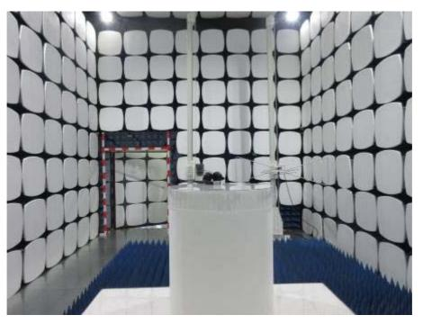
1.1 Radiated Emissions which fall in the restricted bands Test Setup
