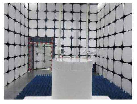
1.1 Radiated Emissions which fall in the restricted bands Test Setup
