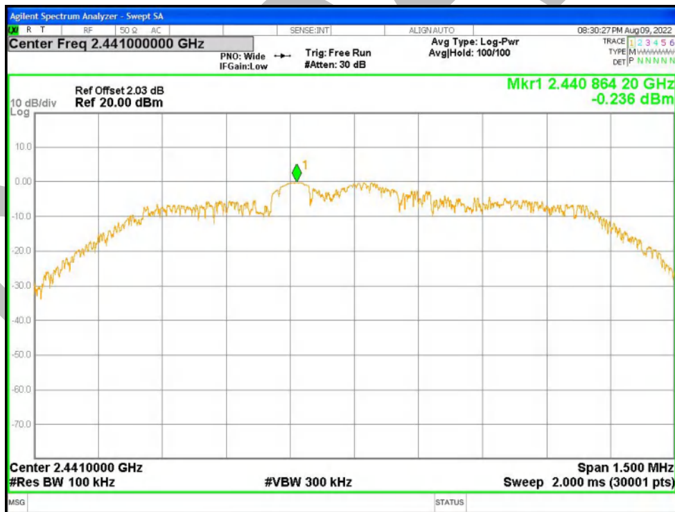
Tx. Spurious NVNT 2-DH1 2441MHz Ant1 Emission
