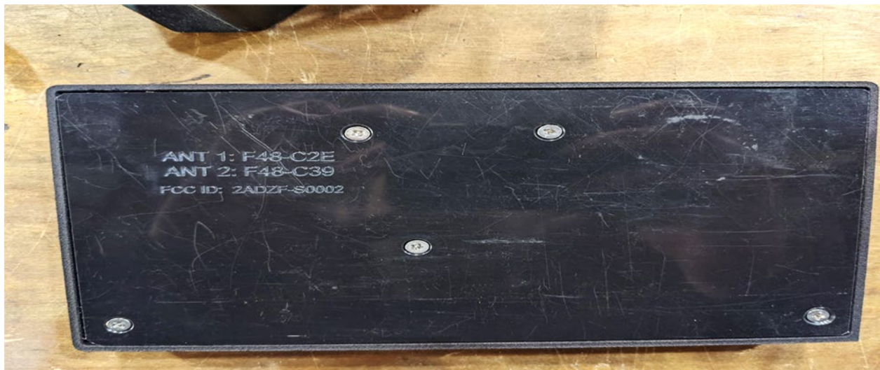
ID Label Location on Bottom of SLR+
