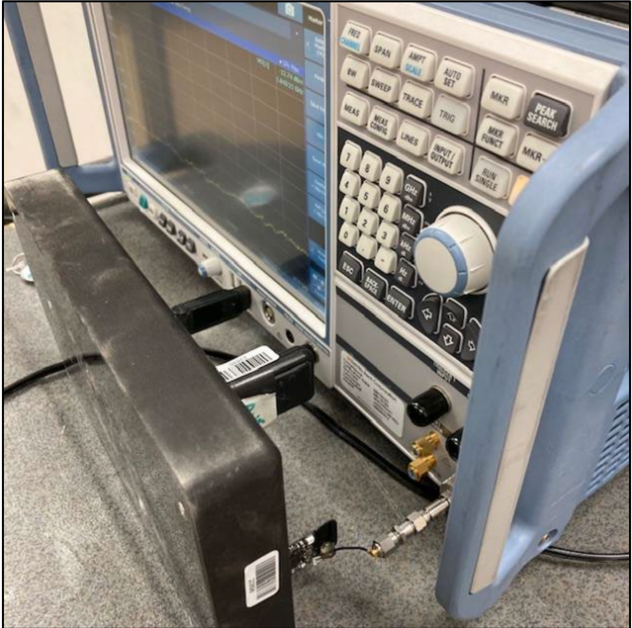
Photograph 5: Conducted Antenna Port
