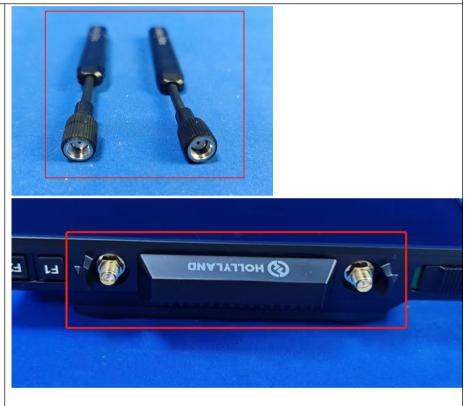
The antenna is internal antenna with ipex connector. The best case gain of the 5G WiFi antenna is 3.77dBi@Band 1, 3.32dBi@Band 4.
