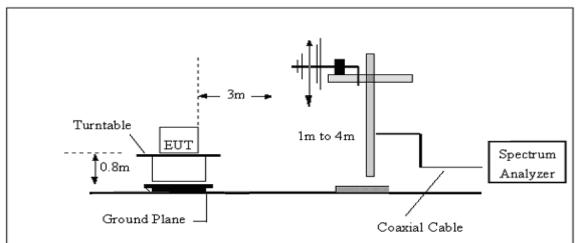
3. Radiated Emission Test-Up Frequency Above 1GHz
