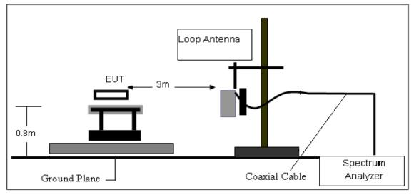
2. Radiated Emission Test-Up Frequency Below1GHz
