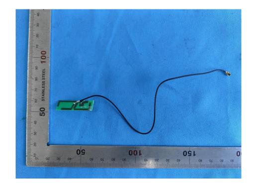
The EUT antenna is PCB antenna. It comply with the standard requirement.
