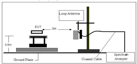
2. Radiated Emission Test-Up Frequency Below1GHz
