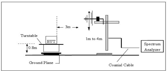
3. Radiated Emission Test-Up Frequency Above 1GHz
