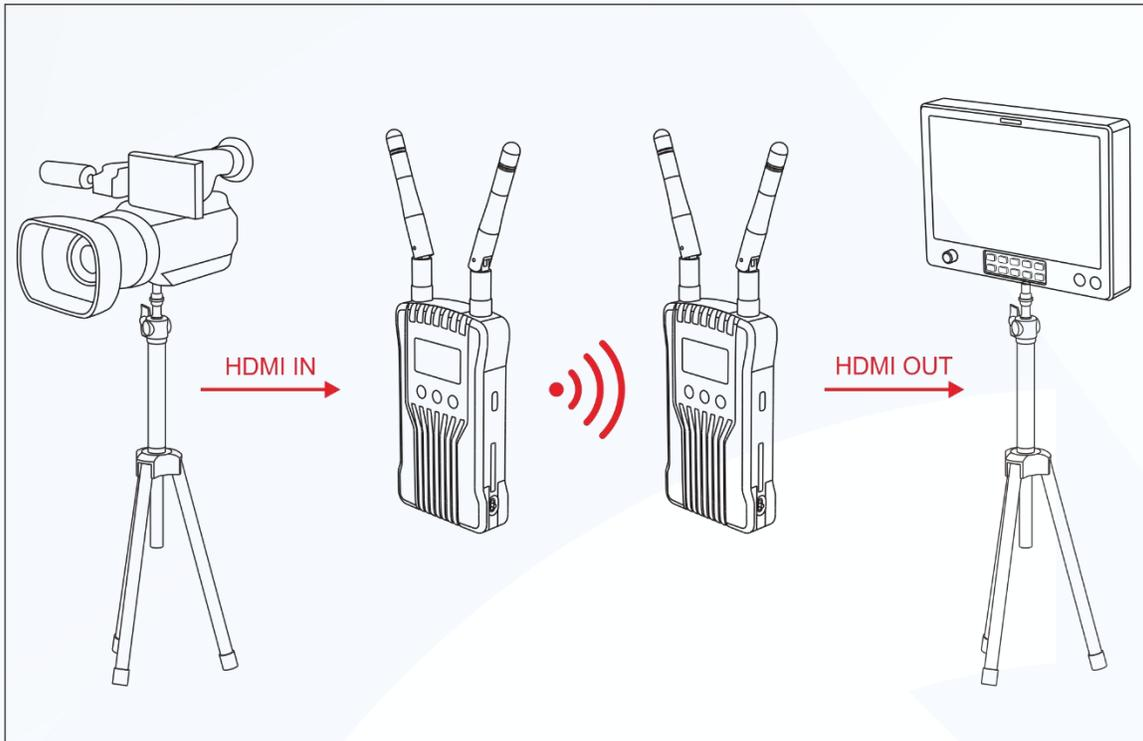
This wireless HD video transmission system uses the latest wireless communication technology, and transmits ultra-low latency HD video transmission. The transmitter supports HDMI Input and HDMI loop out, while the receiver supports dual HDMI output. It is equipped with OLED display screen and supports Smart Terminal Monitoring.
