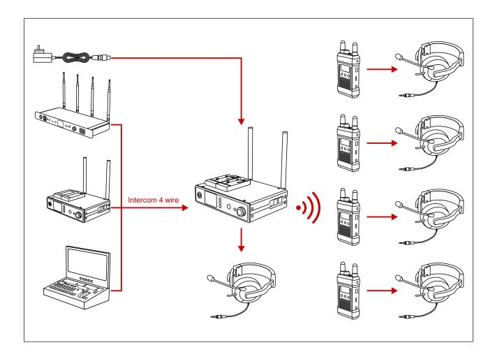
The base station of this wireless full-duplex intercom system supports up to 4 beltpacks. The base station and the beltpacks support dynamic and electret mics. They could be switched by selecting different applications in the menu. The 4-pin audio interface on the base station enables the device to connect with other audio systems, which can increase the quantity of beltpacks and also the wireless communication range.
