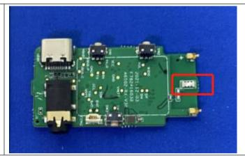
The antenna is Chip antenna. The best case gain of the antenna is 0.1dBi.
