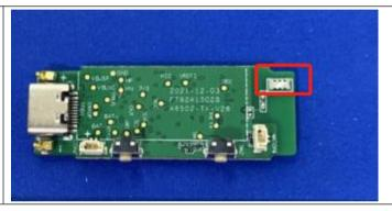
The antenna is Chip antenna. The best case gain of the antenna is 0.1dBi.
