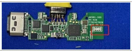
The antenna is Chip antenna. The best case gain of the antenna is 3.18dBi.
