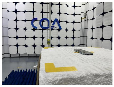
**Conducted Emission Test Setup**
