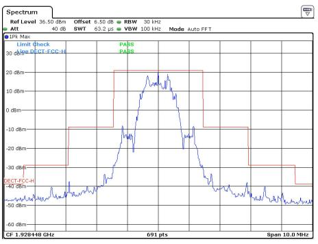
High Channel (Unwanted Emission inside the Sub-band)
