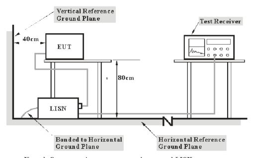
Note: 1. Support units were connected to second LISN. 2. Both of LISNs (AMN) 80 cm from EUT and at the least 80 cm
