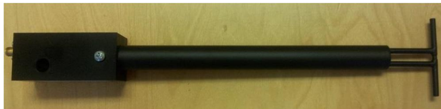
Figure 1 – MVG COMOSAR Validation Dipole
